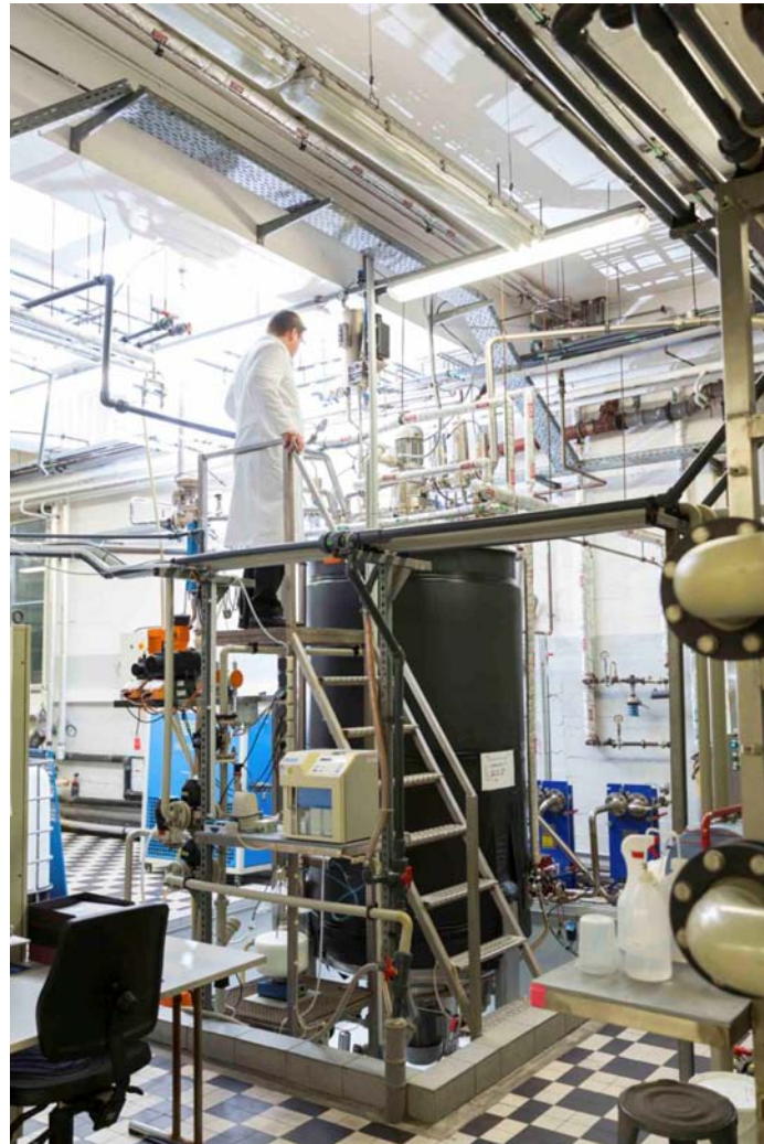
Fig. (1). Bioreactor at the bitop company for the large-scale production of ectoine with the halophilic producer strain H. elongata .
