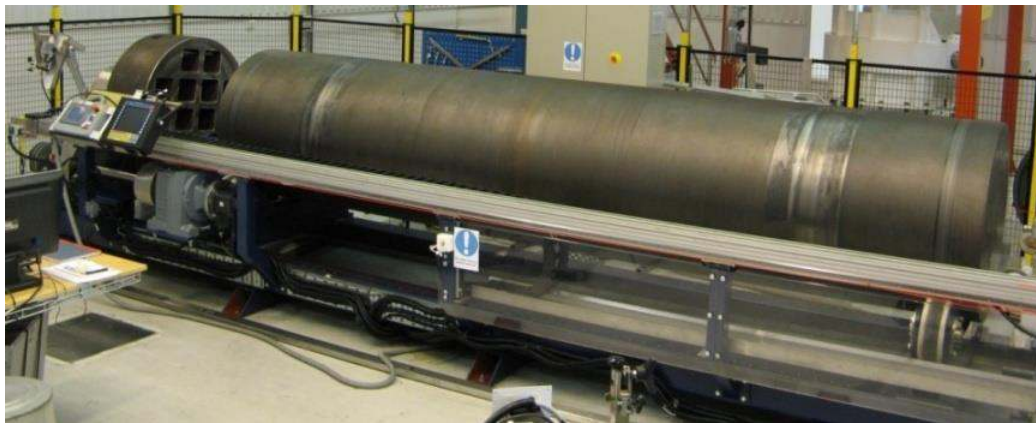
Fig. 6. Manipulator for the cast iron insert with the reference block to the left.
