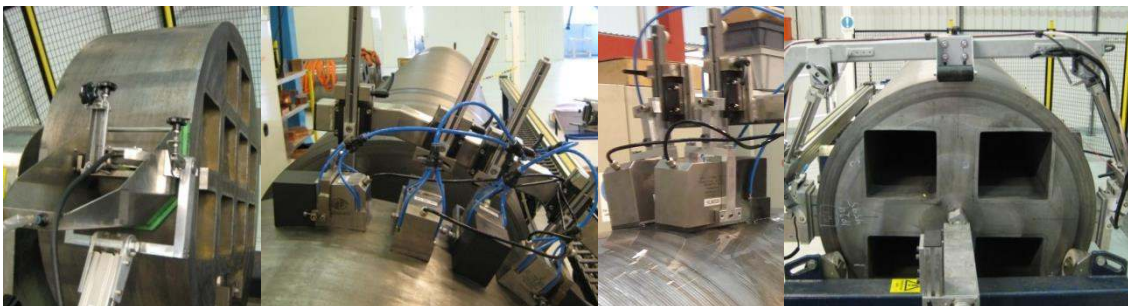
Fig. 9. The different phased array ultrasonic inspection techniques and their associated setups for the insert. Normal incidence local immersion technique (left), two versions of angular shear wave (middle) and transmission techniques (right).
