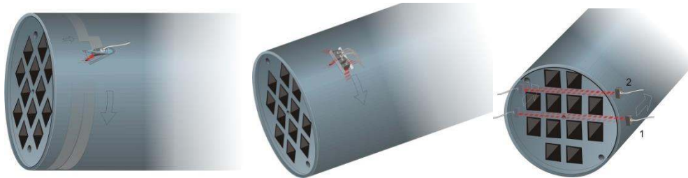
Fig. 8. The different phased array ultrasonic inspection techniques for the insert. Normal incidence local immersion (left), angular shear wave (middle) and transmission (right).
