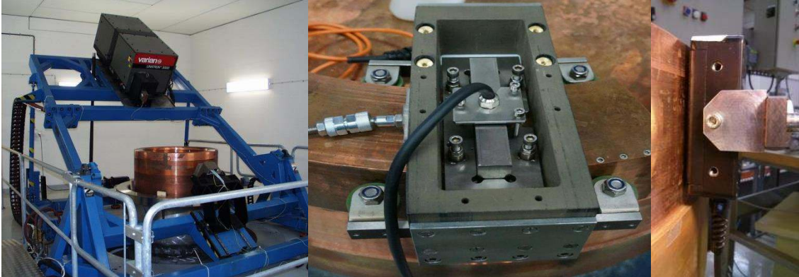
Fig. 12. Inspection of the copper friction stir weld: Digital X-rays (left), phased array ultrasonics (middle) and eddy current array (right)
