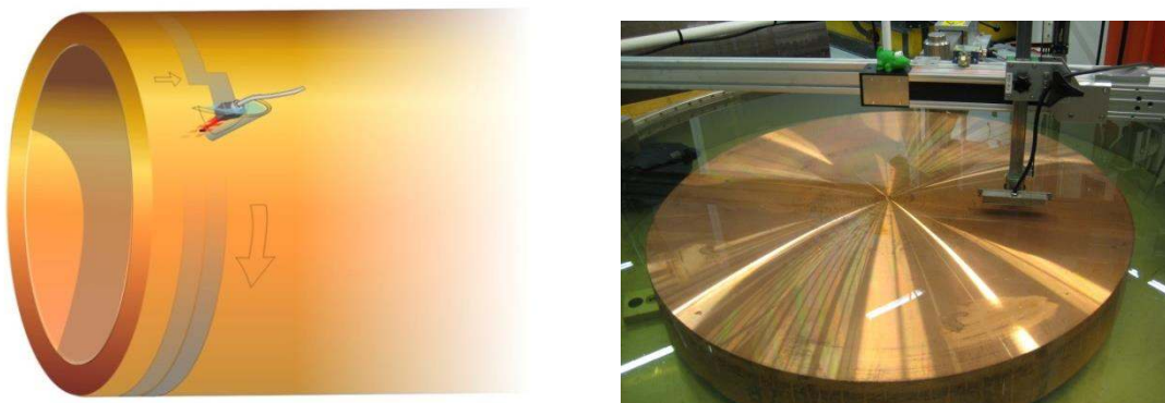
Fig. 11. Local immersion ultrasonic inspection of the copper tube (left) and ultrasonic immersion inspection of the copper lid/base (right).
