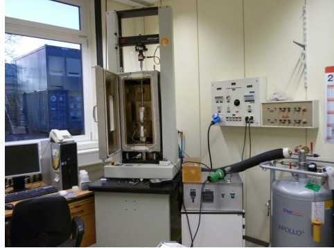
Figure 3.1.: Setup for cyclic thermomechanical measurements.
