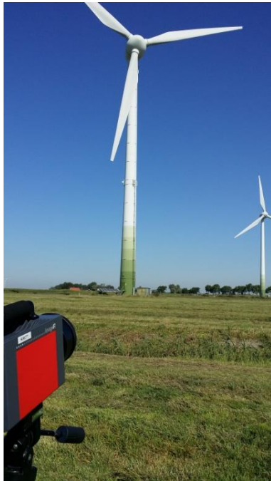
Fig. 1: onsite investigation of a rotating wind turbine at sunny weather, distance of about 250 m to the hub
