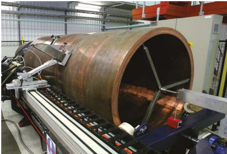
Figure 12: The ultrasonic equipment mounted onto a rotating component (Source: SKB; with permission)
