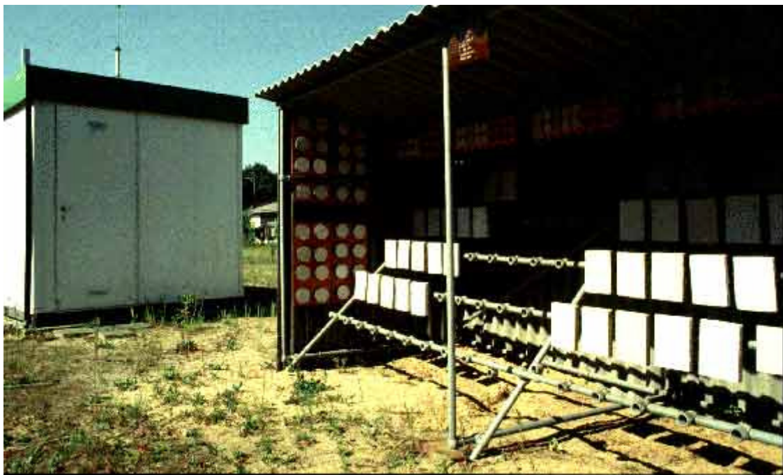
Fig. 5. Rack facing south for exposing rendering specimens to ambient atmosphere (Air monitoring station shown at left in background)
