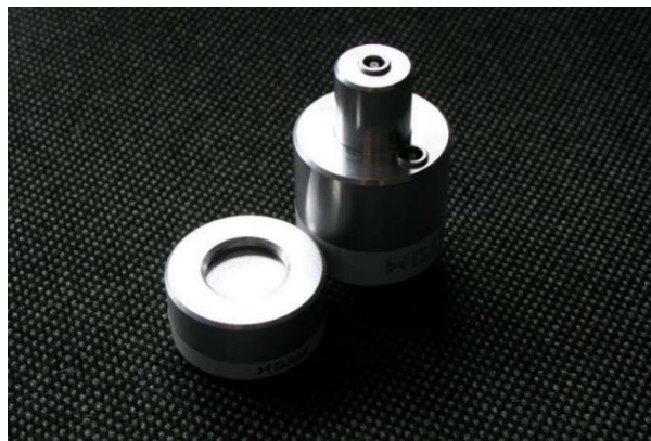
Fig. 1. Focusing transducer for air-coupled ultrasonic testing based on cellular polypropylene (front) with electric matching unit (background)
