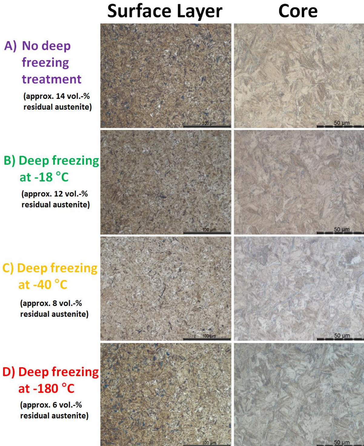
Figure 3.2: Light microscope images of the surface layer and core of heat treated 20MnCr5.
