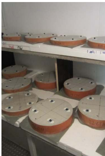
Figure 1. Photo of the samples in the climate chamber at T = 23^{\circ}\text{C} , rH = 50\% (left). Results of the destructive Darr and CM methods measuring screed moisture. CA indicates anhydrite based screed and CT cement based screed (right).
