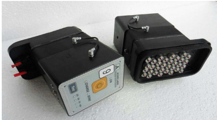
Figure 1: One ultrasonic unit of the LAUS system. Each Module consists of 32 dry point contact transducers which are spring loaded and ensure the mechanical contact to the concrete surface. It is fixed using a vacuum case. Additionally there is a electronic module for data transfer.
