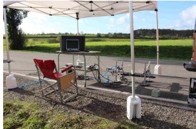
Figure 10: Measurement on highway B35 near Illingen (Germany) with the automatic scanner system [1]
