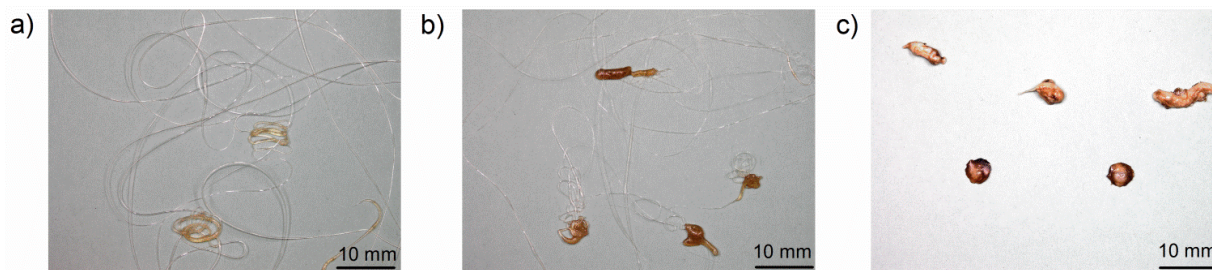
Figure 8. (a) Melt flow of PA 6 HB at a furnace temperature of 400 °C; (b) melt flow and drops of PA 6 HB at 550 °C; and (c) drop pathway of PA 6 V-2 at 550 °C.
