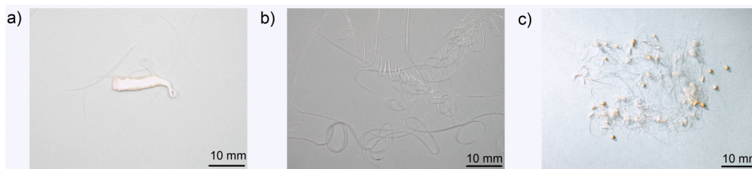
Figure 4. (a) Partly molten piece falling down of PBT V-2 at a furnace temperature of 500 °C; (b) melt flow material of PBT HB at 400 °C; (c) melt flow and dripping of PBT HB at 650 °C.
