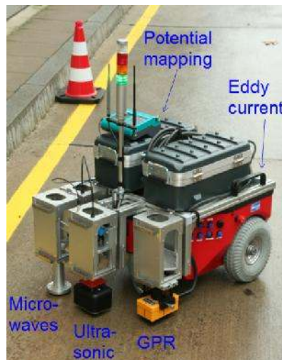
Figure 1. The BetoScan robot system with NDT sensors
