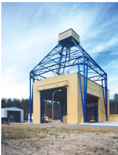
Fig. 7 Drop test facility (200 tons lifting capacity) on BAM TTS
