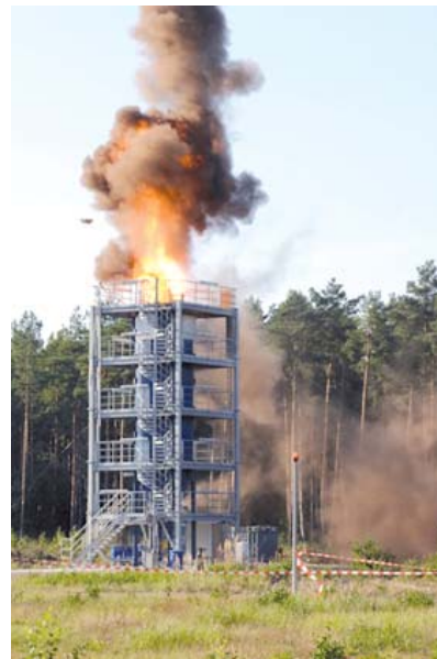
Fig. 5 Dust explosions and devices such as pressure relief openings may be investigated in the test silo on BAM TTS. Filling volume 50 m 3 , pneumatic charging
