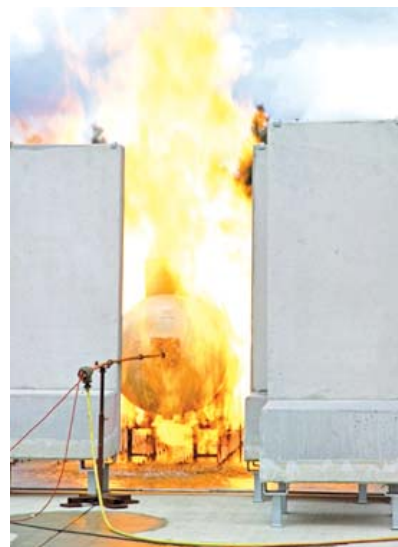
Fig 6 Fire test of a dangerous goods container in the fire test rig for destructive testing. The wind shielding plate has been removed for demonstration
