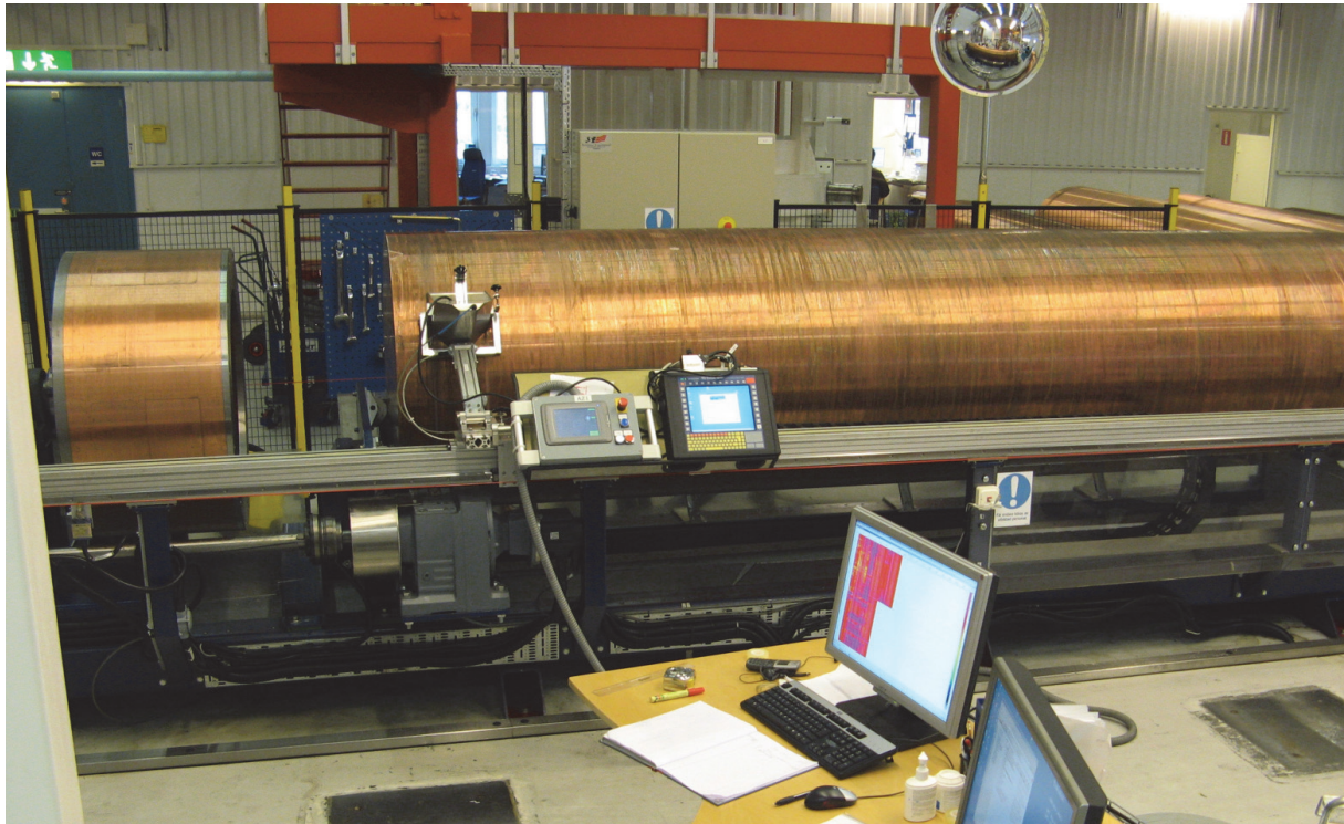
Figure 8: Mechanized Inspection of the copper tube; UT equipment; Probe 128 elements, linear array, pitch 1 mm, width in passive direction 16 mm
