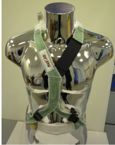
Figure 24. Sensing harness containing fiber optic sensors for the monitoring of patients under MRI. A thoracic respiration sensor is integrated in the black part (upper right); an abdominal respiration sensor is integrated in the white part (lower middle).
