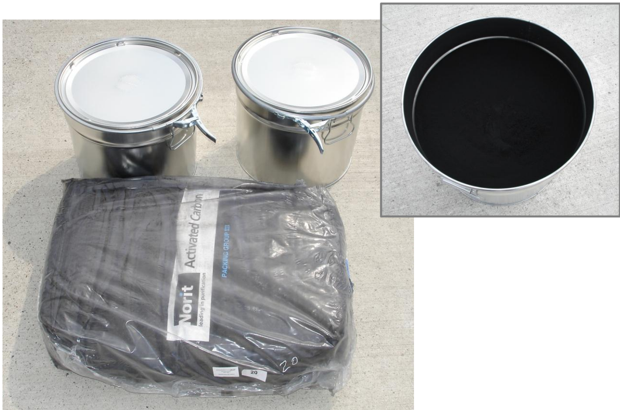
Figure 4-2: Interlaboratory test sample “Carbon Black, Norit CN4”: bag from the supplier and 2 hobo-bucks (20 l, Dosen-Zentrale Züchner GmbH, Köln) for one participant of the interlaboratory test
