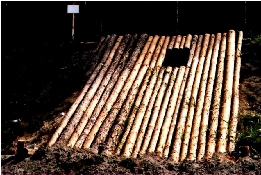
Fig. 5.11: Camera at the earth embankment; distance to the fire stand approx. 200 m
