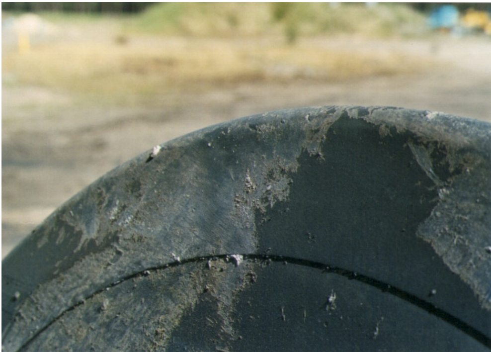
Fig. 25: Traces of concrete on the bottom edge of the Castor
