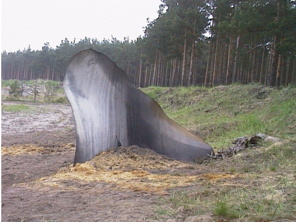
Fig. 17: Position of the jacket section (1) after the test
