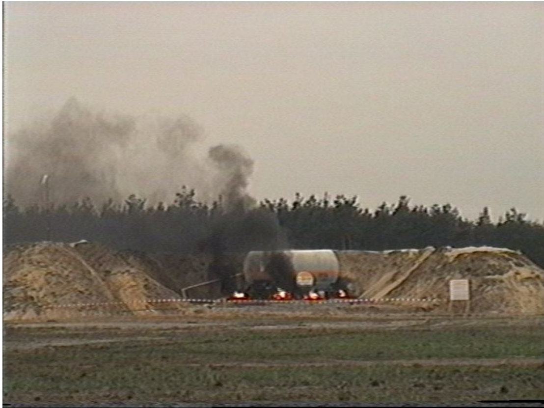
Fig. 8: Triggering the ignition devices
