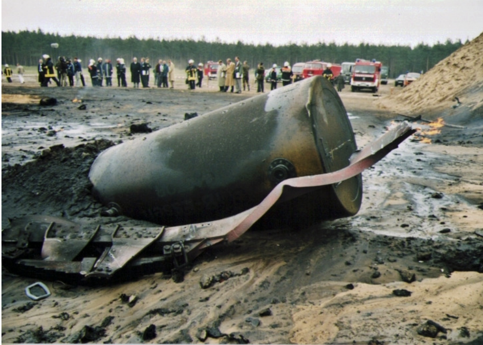
Fig. 24: Position of the Castor container after the test
