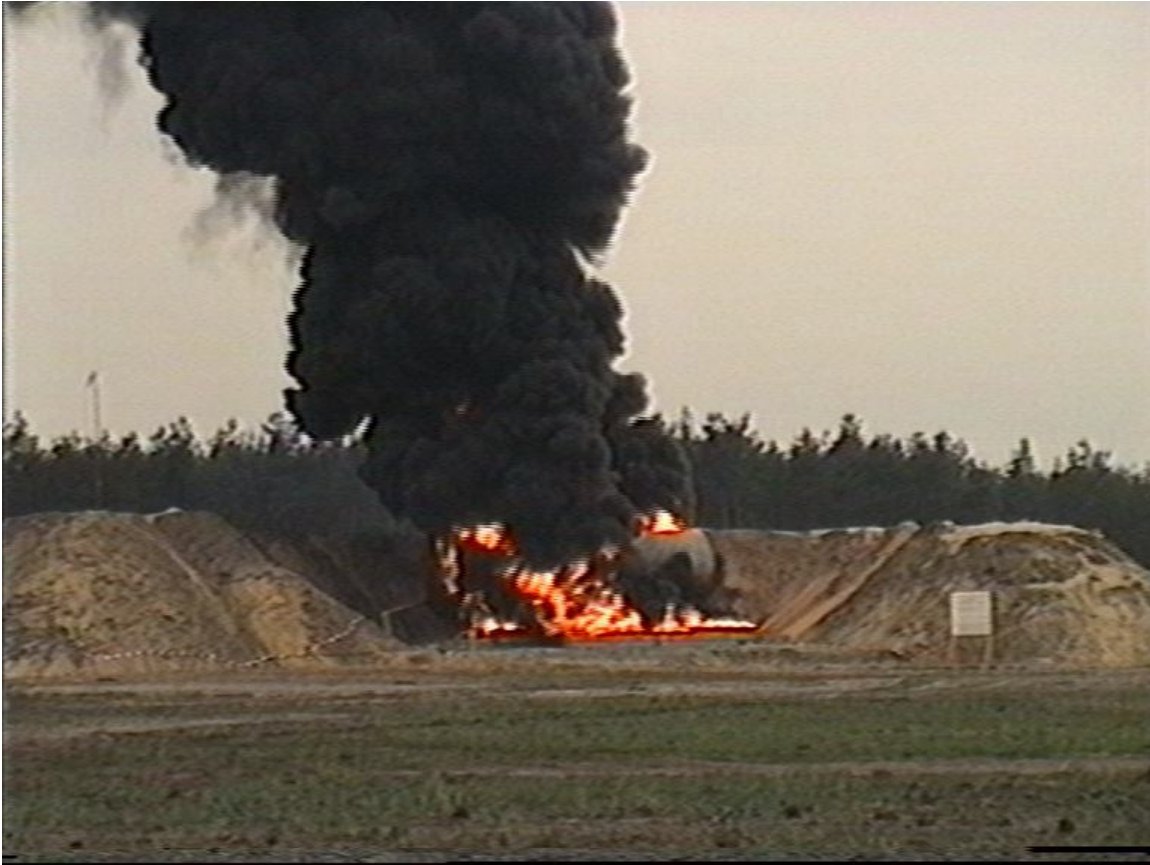
Fig. 10: Improved flame envelopment towards the end of the test
