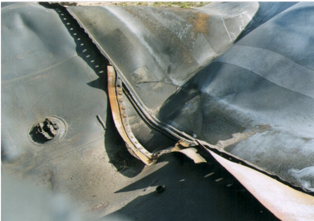
Fig 27: Dent in tank car's jacket, the point at which it came into contact with the Castor
