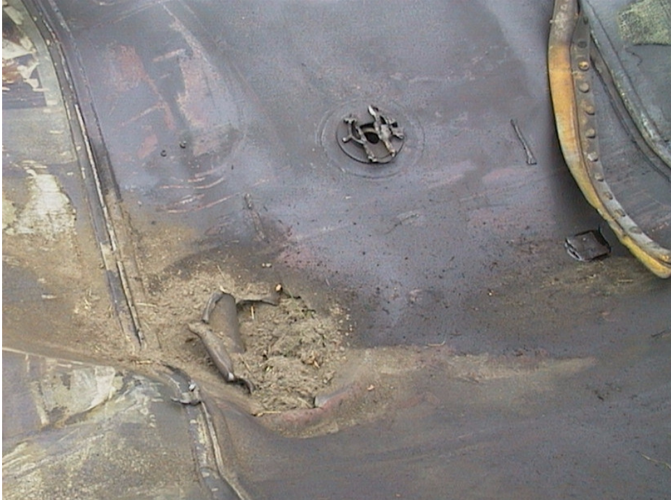
Fig. 28: Opening in the jacket due to contact with Castor's support
