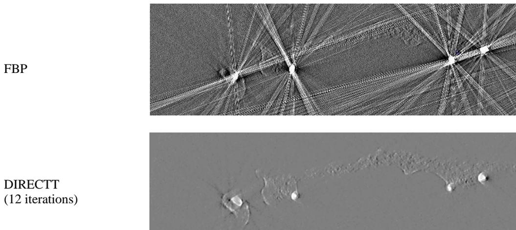
**Fig. 4.** Comparison of Filtered Backprojection (top, no data pre-processing) to the DIRECTT iteration (bottom).
