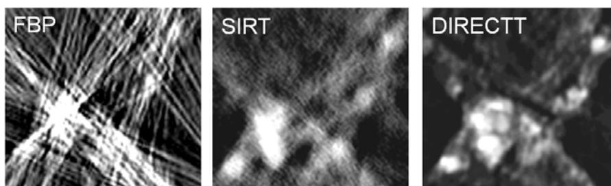
**Fig. 5.** Quality comparison of different reconstruction algorithms at the example of a catalyst particle agglomerate (reconstruction detail). The dominant streak artifacts appearing in the FBP (left) are purged in the SIRT (Simultaneous Iterative Reconstruction Technique, center) result. However, the central large particle is resolved by application of the DIRECTT algorithm (right) into four separate particles, exclusively.
