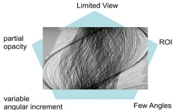
**Fig. 3.** Simultaneously occurring restrictions of data sets in electron tomography.
