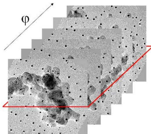
**Fig. 2.** Series of projections (TEM images) with an indicated plane containing planar sinogram (red). The strongly absorbing gold markers appear black. The small catalyst particles are distributed on (and inside) the cloddy carbon black supports.
