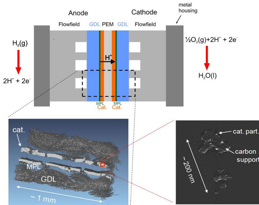
**Fig. 1.** Schematic set-up and functional principle of a PEM fuel cell (top), magnification of the MEA (Metal Electrode Assembly, bottom left) and components of the catalyst layer (single reconstructed electron CT slice, bottom right); PEM: polymer electrolyte membrane, MPL: Micro porous Layer, GDL: gas diffusion layer.
