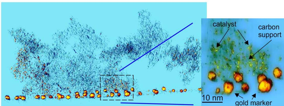
**Fig. 6.** 3D visualization of Ru catalyst nano particles and magnified detail at about 1 nm spatial resolution; dominant 3–8 nm Au markers on cloddy carbon black supports.
