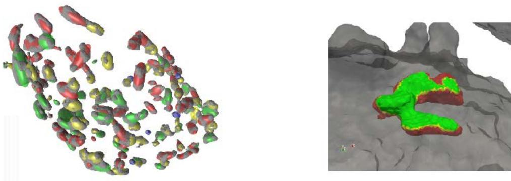
**Fig. 7.** Examples of analyzing the reconstructed data: left: catalyst particles approximated by ellipsoids (shape, orientation), right: partial embedding of a catalyst particle on carbon black support (reactive surface (green), buried surface (ruby)).
