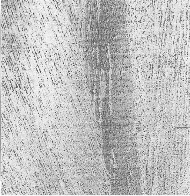
Figure 1.19: Acoustic micrograph of a X 6 CrNi 18 11 weld metal cross section, 1mm × 1mm, 1 GHz (Haubold 1999 [74])
