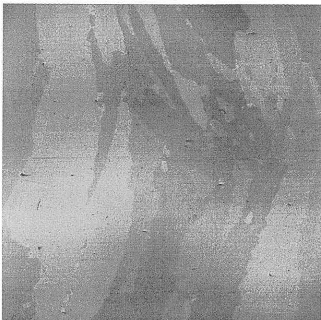
Figure 1.21: Acoustic micrograph of Nickel based alloy NiCr 19 Nb weld metal, transverse weld section, 1mm × 1mm, 1 GHz (Haubold 1999 [74])
