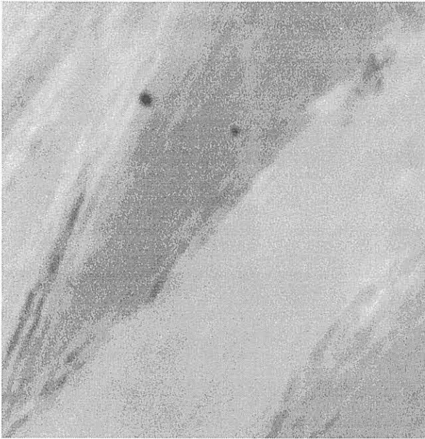
Figure 1.23: Acoustic micrograph of a X 2 CrNi 19 9 weld metal cross section, with increased Ni-content, 1mm × 1mm, as in fig. 1.20 but 100 MHz (Haubold 1999 [74])
