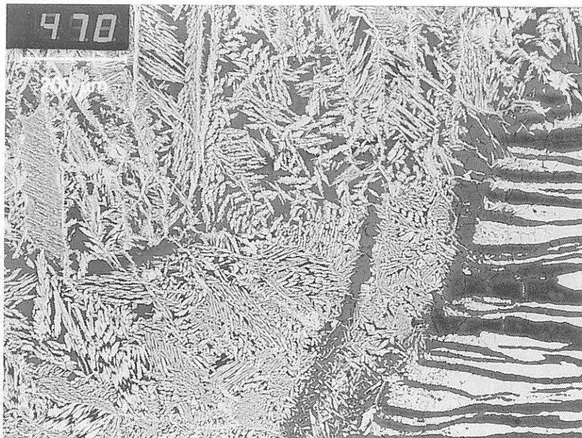
Figure 1.6: Duplex weld metal; cross section; detail at the fusion face; base metal: ferrite and austenite ( \alpha/\gamma )-solid solution; weld metal: Widmannstätten structure; same weld as in fig. 1.5 (Bauer 1999 [46])
