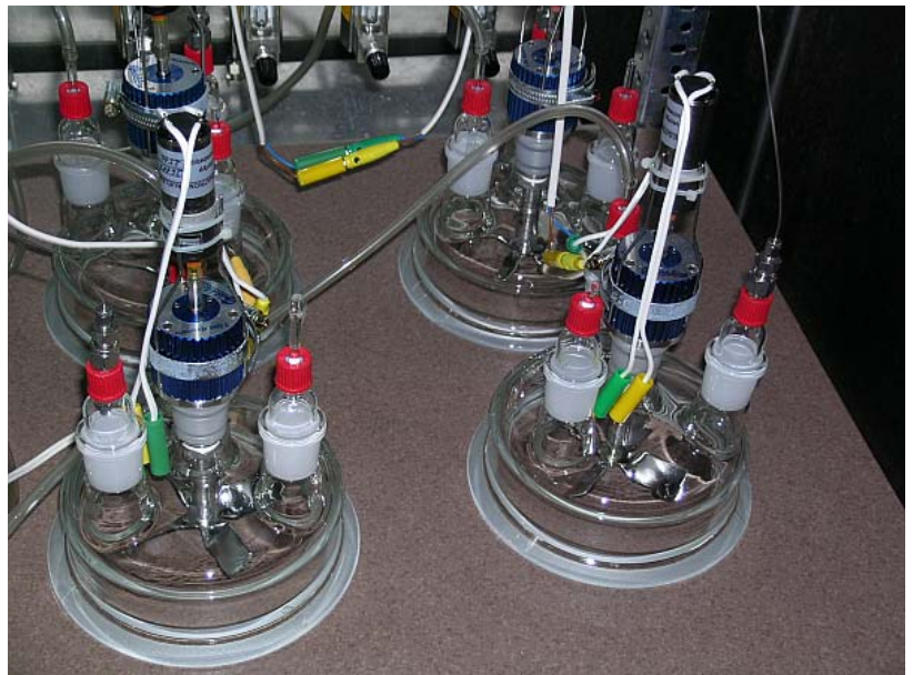
Figure 35: Four emission cells placed on a floor covering to test inhomogeneities within the sample.
