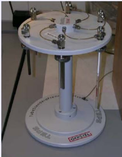
Adding 20 ng cyclodecane on the sampling tubes with 5 min N_2 -stream
