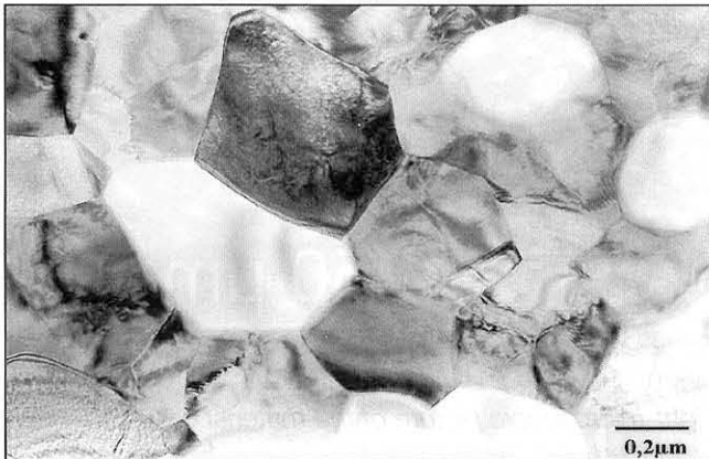
Fig. 11 TEM picture of the structure of the material HIP-ZrO 2
