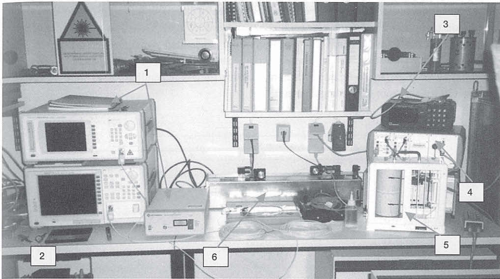
Figure 4.2: Measurement set-up: 1 - light sources; 2 - OSA; 3 – elongation meter; 4 – controlling unit of the tensile test machine; 5 – moisture and temperature meter; 6 – tensile test machine.
