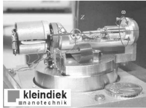
(b) Nanopositioning stage on SEM stage
