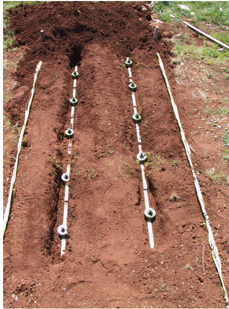
Figure 7.2: Placement of targets before their burial for maximum detection height measurements. The boards help to control the depth of the targets.
