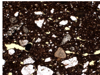
Figure A.4: Thin section images of limestone, sand-limestone (type KS) and brick (type Ha) made with a polarizing microscope using plain polarizing light.
