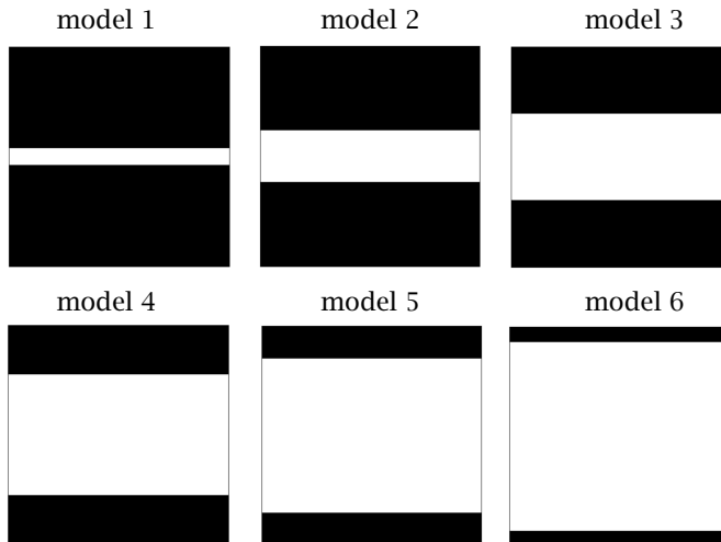
Figure 6.14: Model set with varying porosities \Phi . From model 1 (top left) to model 6 (bottom right) \Phi takes the values 0.08, 0.23, 0.39, 0.55, 0.70, 0.85.
