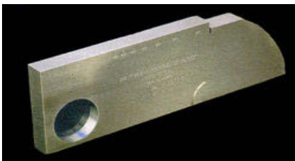
Fig. 4.11: IIW Type US-1 calibration block
