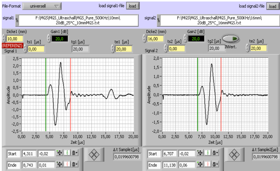
Fig. 4.8: Recorded A-Scans for 10 and 16 mm epoxy samples. Oscilloscope settings were 20 \mu s time window and amplification 20 dB for both samples.
