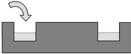
Figure 28: Schematic set-up of ring casting test (cross-section).
