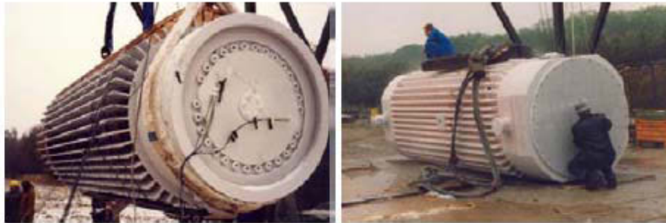
Figure 3.1: Prototypes of Fuel Element Transport Casks TN900 (left) and CASTOR ® Ic (right) Before or After a 9-m Drop Test
