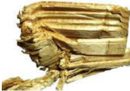
Figure 4.20: Kinked Wood Fiber Bundle Using the Example of Fir Wood Compressed in the Axial Direction (Experiment M. Neumann, BAM, 2007)
