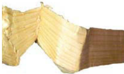
Figure 4.19: Kinked Wood Fiber Bundle Using the Example of a Piece of Fir Wood Compressed in the Axial Direction During a 9.0-m Drop in a Shock-Absorbing Part
