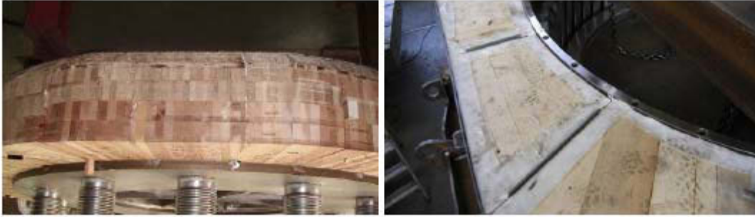
Figure 2.6: Filling of Shock Absorbers Attached to the Cask Ends (left: MHi shock absorber, right: GNS CONSTOR ® shock absorber)
