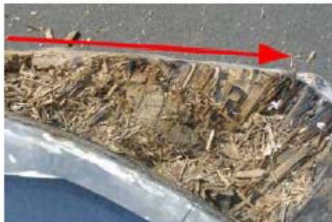
Figure 4.21: Shock-Absorber Filling of the MSF69BG® Bottom Shock Absorber after a 9.3-m Slap Down Drop, View from the Cask
