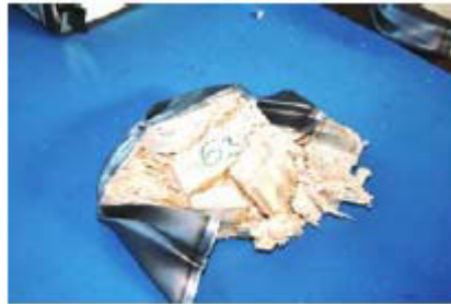
Figure 4.30: Torn Sheet-Metal Jacket in a Sample with Axially Stressed Wood (V63, ml300)
