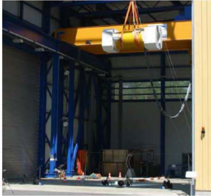
Figure 4.9: Performance of Shock Absorber Testing Drop Test in the Horizontal Drop Position on 069/271/2006
