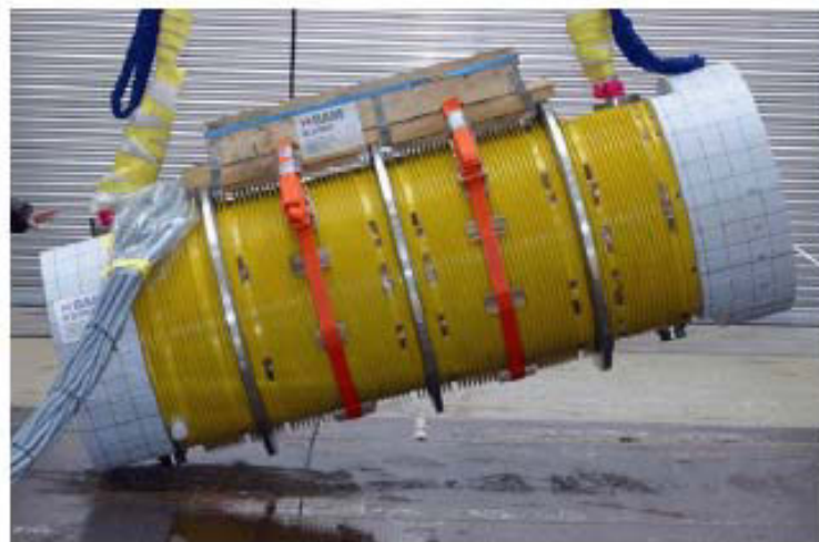
Figure 3.3: 1:2 Model CASTOR ® HAW TB2 Before a Slap Down Drop Test at the Drop Test Facility of the BAM
