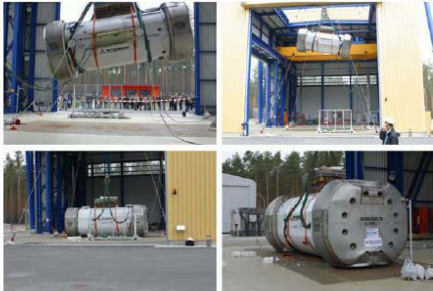
Figure 4.7: Performance of the MSF69BG® Drop Test in the Slap Down Drop Position on 09/24/2004
