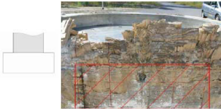
Figure 4.22: Shock-Absorber Filling of the MSF69BG ® Bottom Shock Absorber after a 9.3-m Slap Down Drop After Removal of the Outer Sheet-Metal Pieces, Subdivision into Zones with Cavity Compression and Fiber Delamination
