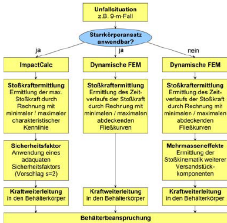
Figure 7.2: Scheme Showing Possible Procedures To Be Used for Mathematical Data Evidencing the Accident Safety of Transport Casks Holding Radioactive Substances
