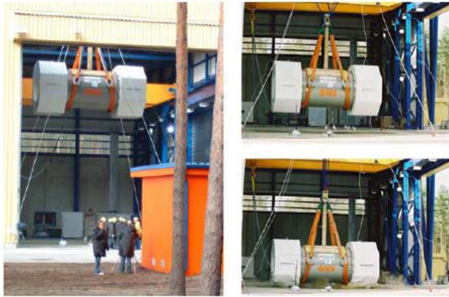
Figure 4.8: Performance of the CONSTOR ® V/TC Drop Test in the Horizontal Drop Position on 09/21/2004
