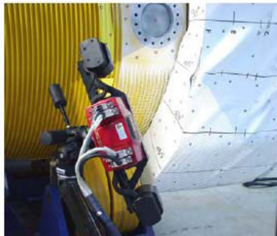
Figure 4.14: Measurement Setup for Measuring the Shock-Absorbing Part During the Shock-Absorber Test Using the Strip Projection Method
