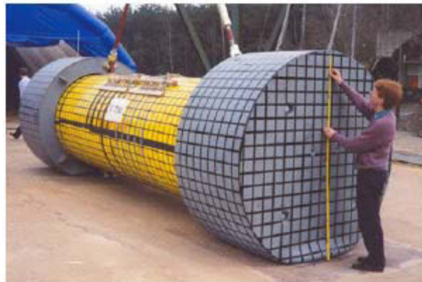
Figure 2.5: Round, Wood-Filled Shock Absorbers on the GNS (Gesellschaft für Nuklearsysteme mbH) POLLUX ® Cask After 9-m Horizontal Drop
