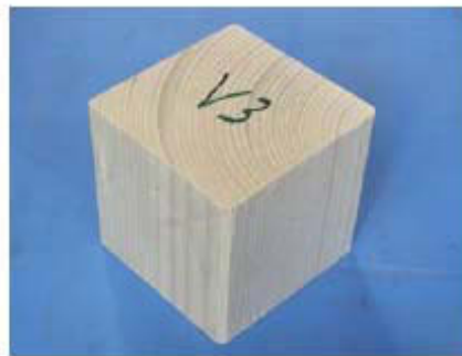
Figure 4.25: Cubic Sample Made of Fir Wood with an Edge Length of 100 mm
