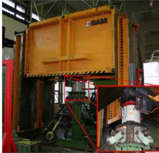
Figure 4.27: Servohydraulic Impulse Test Stand of BAM
