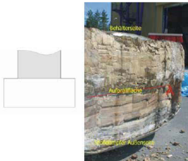
Figure 4.18: Shock-Absorber Filling of the MSF69BG ® Bottom Shock Absorber after a 9.3-m Slap Down Drop, Viewed Diagonally from the Direction of the Foundation
