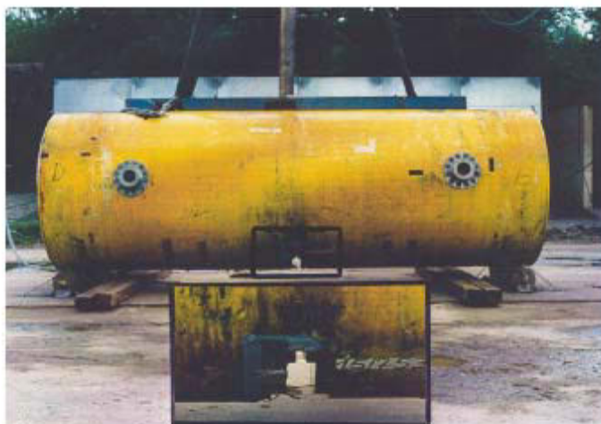
Figure 2.9: CASTOR ® VHLW ® Cask with a 120-mm-Deep Flaw in the 260-mm-Thick Wall, Impact Upon a Steel Roller Bearing
