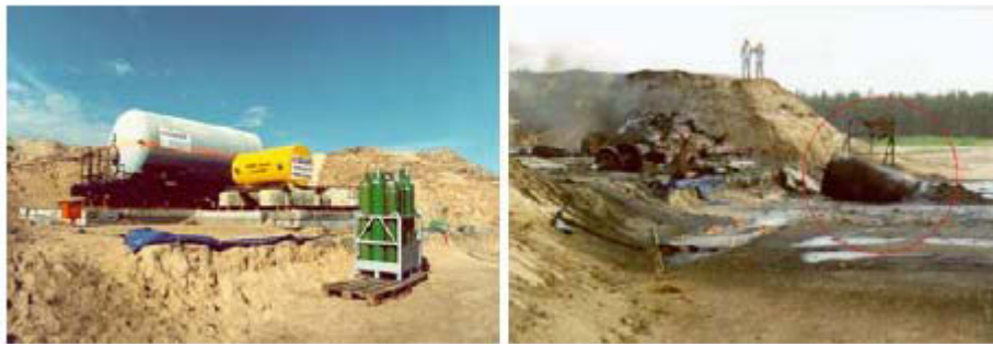
Figure 2.10: Fire Test with a Railroad Tank Car and a CASTOR ® THTR/AVR ® according to [DPH99] Before (left) and After the Experiment (right).
