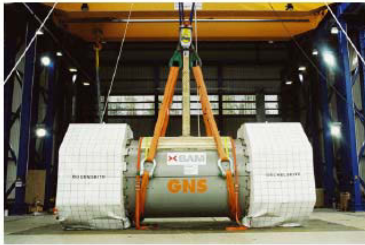
Figure 3.2: 9-m Drop Test with a CONSTOR ® V/TC Experimental Cask on the Original Scale at the Drop Test Facility of the BAM
