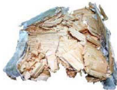
Figure 4.26: Cubic Sample Made of Fir Wood with Lateral Expansion Inhibition Destroyed During Test Consisting of Glass-Fiber Reinforced Synthetic Substance
