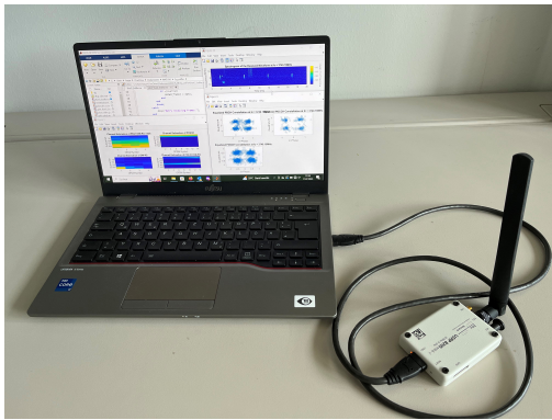
Fig. 2. Hardware setup for 5G monitoring
